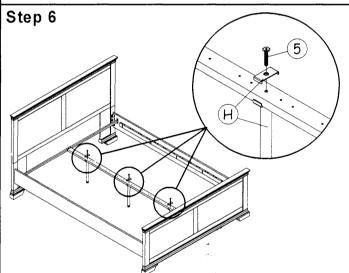
Fix bed support legs as shown and tighten all bolts.
