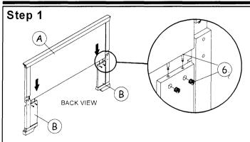
Fix head bottom leg left & right tio the head board top with minifix '6' as shown.
