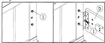
Fix bolts '1' (upper & lower bolts) into position on wood leg as show. After that hook the side rail to the bolt and fix center bolts '1' as shown.
