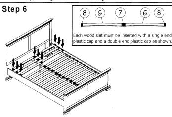
Once both wood slats have been inserted with the plastic caps, fix it on the wood side rails and center bar by pressing it accordingly to the default holes. Ensure the plastic cap's pin is aimed to the hole.
