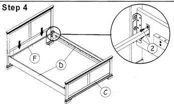
Fix cross bar 'F' to the side rail with bolts '2' as shown.
