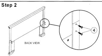
Fix bolts '4' to the headboard top and head bottom leg as shown.
